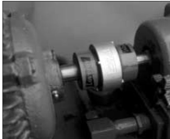
Step 4 Twist locking ring to secure.
