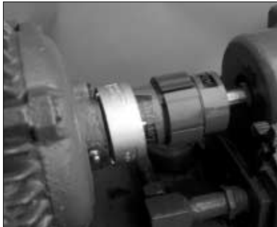
Step 3 Slide locking ring over element.
