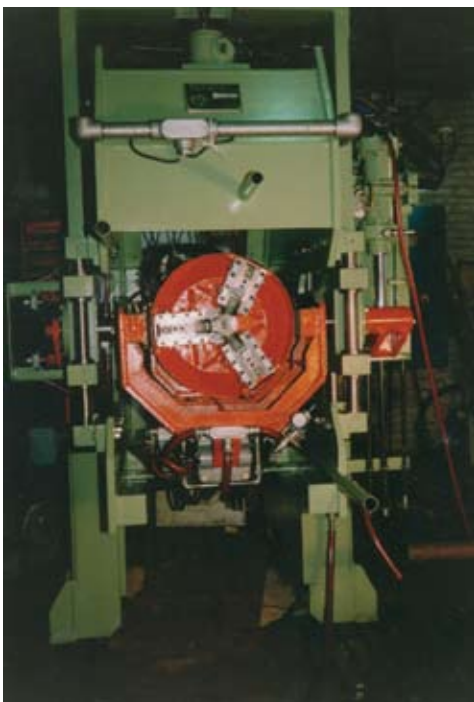
Robot for applying of screw protection in seamless tubes, built for Siderca, from Techint group
